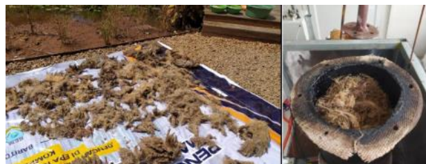
Figure 1. Production of liquid smoke: a. Oil palm dried bunches (EFB), b. EFB in pyrolysator
